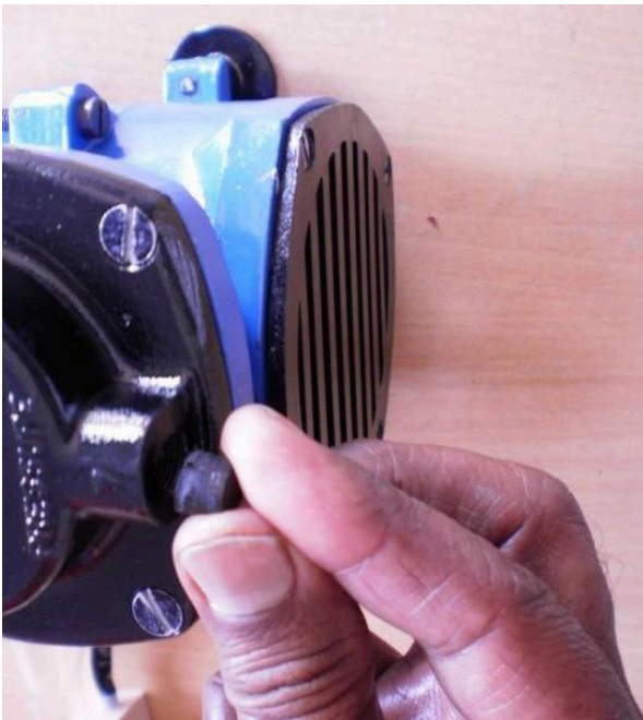
Remove Cap from Vacuum Pump Inlet
