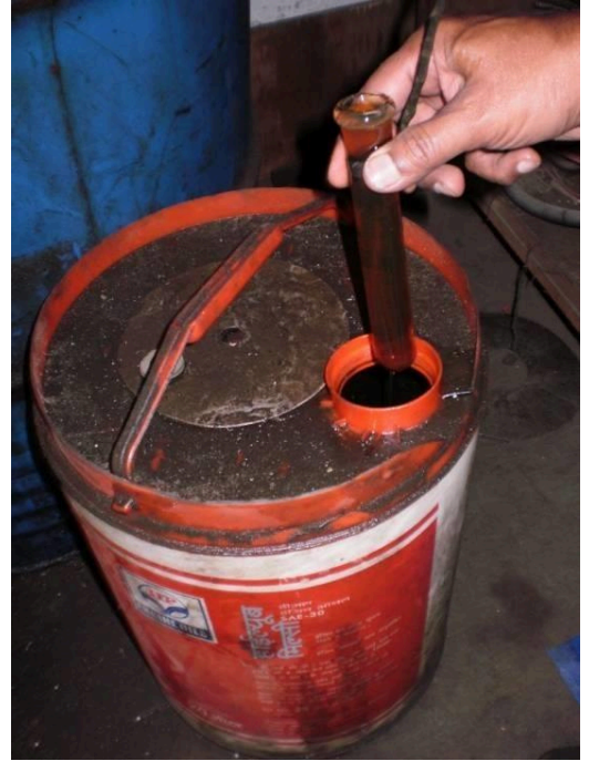
Clamp Funnel on the Base Take Oil Sample in Test Tu
