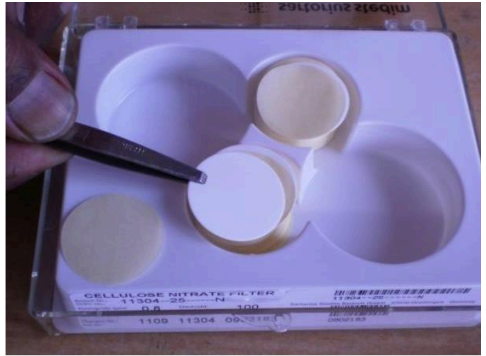
Carefully Lift Test patch. (discard the yellow Cover paper)
