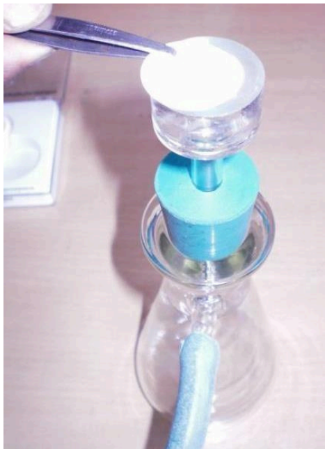
Place Test Patch on Porous Base
