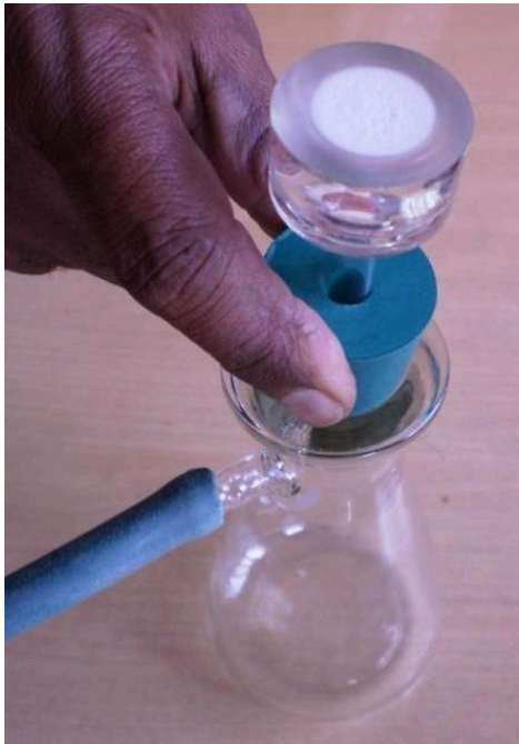
Fit porous Base to Flask
