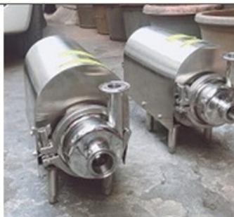
SS SANITARY PUMPS
